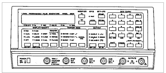
Figure 3-1. Front Panel Controls, Indicators and Connectors
