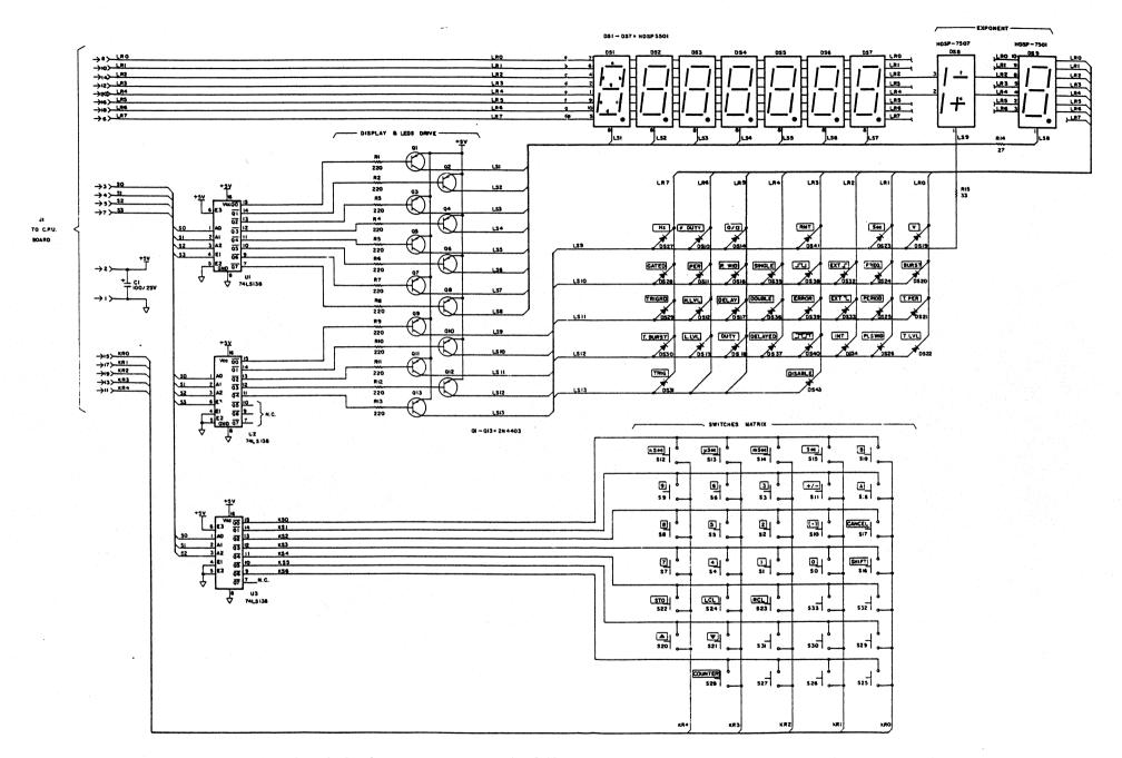
9-13 Display Board - Schematic Drawing
