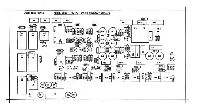
9-12 Output Amplifier Board - Assembly Drawing
