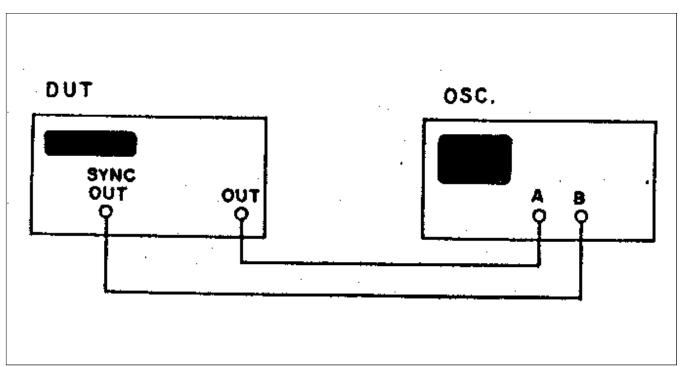
Figure 7-3. System Delays Adjustment.
