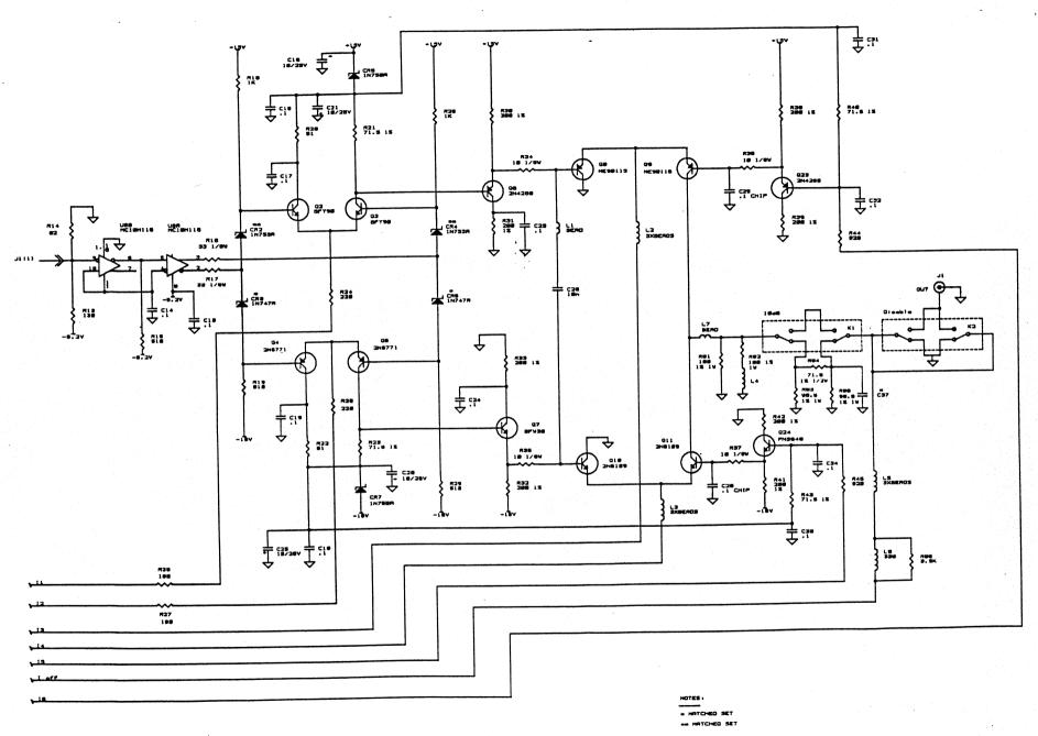
9-10 Output Amplifier Board Part 1 - Schematic Drawing
