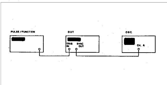
Figure 7-1. Trigger Input Sensitivity Adjustment.
