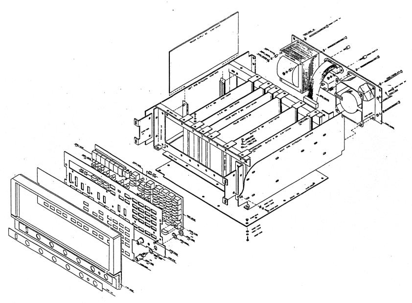
Figure 8-1. Model 8600 - Exploded View
